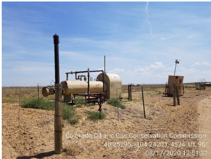
Photo 1 – Separator and Gas Meter House, Weeds
