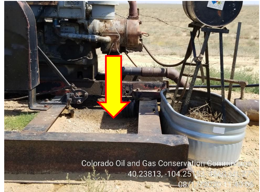
Photo 10 – Stained Soil at Gas Engine
