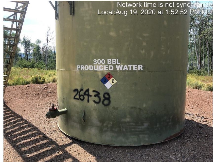
Photo #1757 Tank missing operators name and contact phone number.
