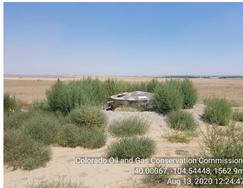
Photo 10 produced water tank. WEEDS and NFPA placards faded and tank volume faded.
