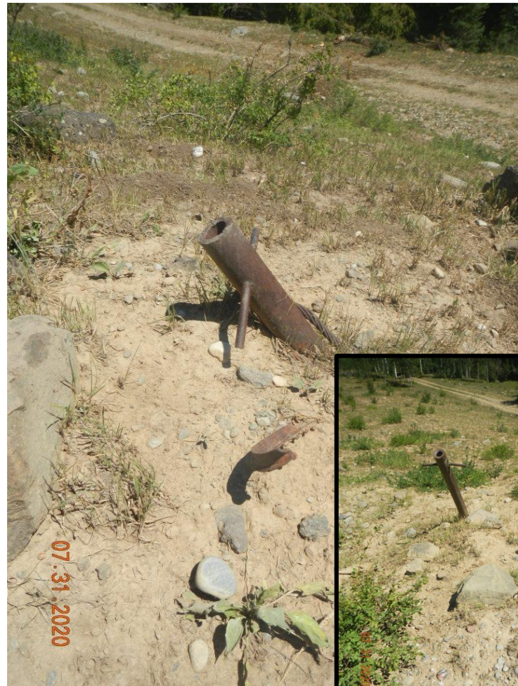
Photo#10: Anchors not Marked.
