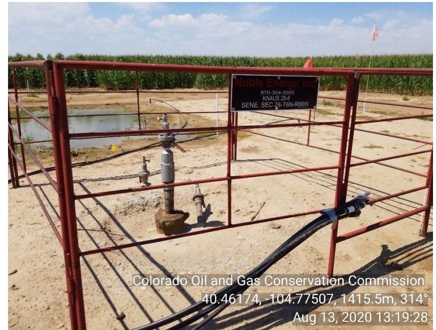
Photo 2: Wellhead; equipment removed
