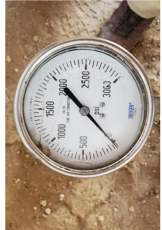
Photo 3 Casing Pressure Gauge
