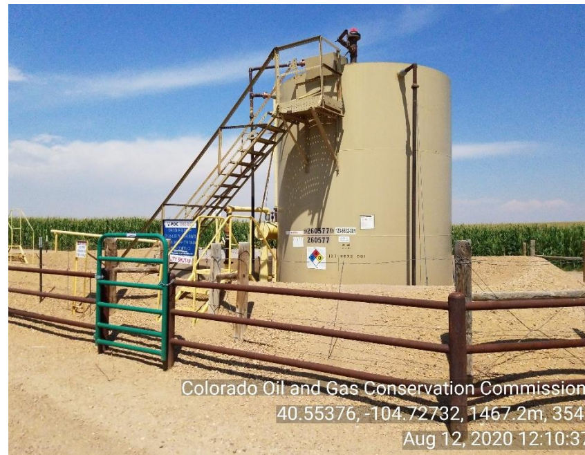
Photo 4: Tank Battery
