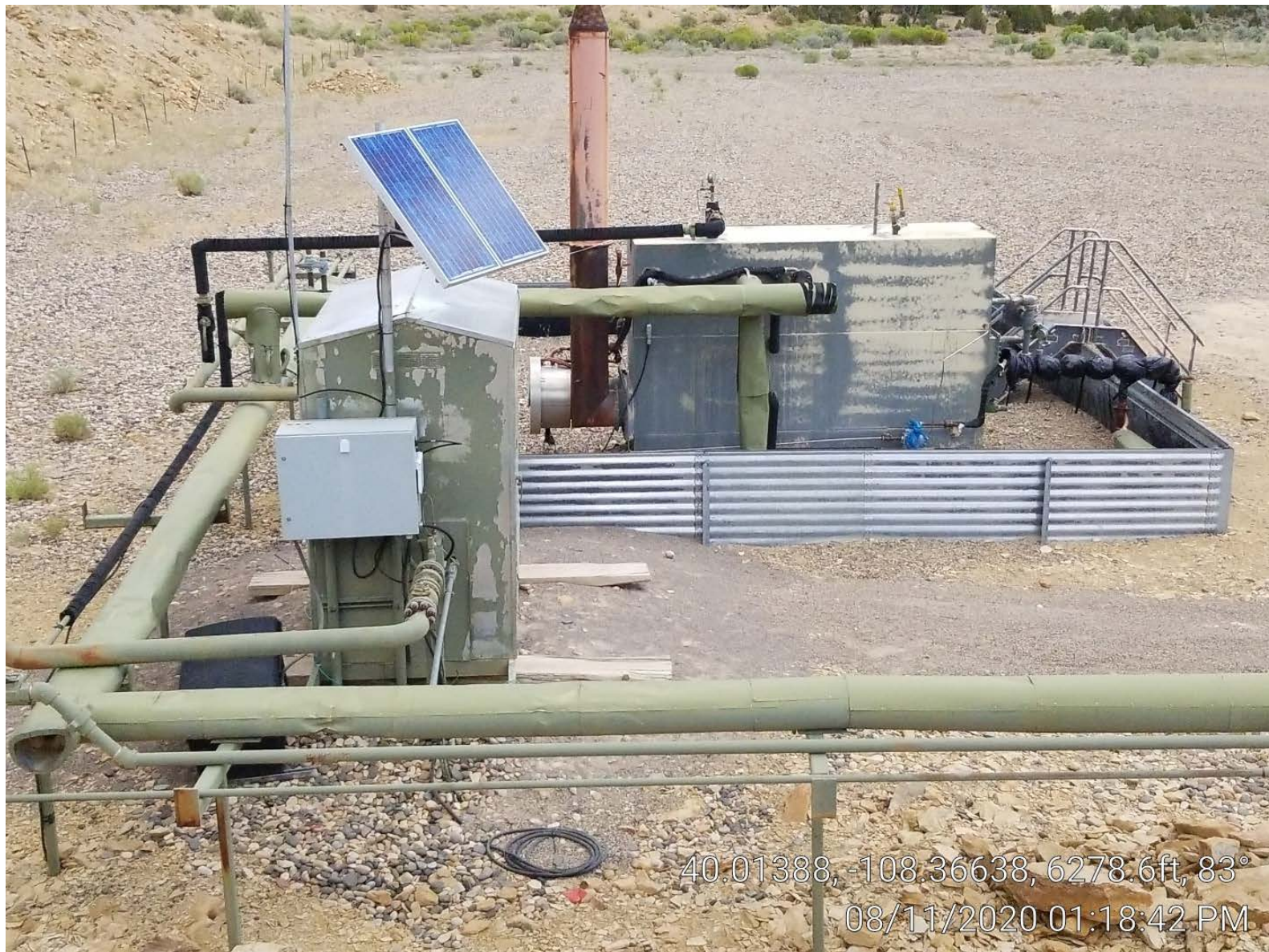
Photo 3. Meter building & separator.
