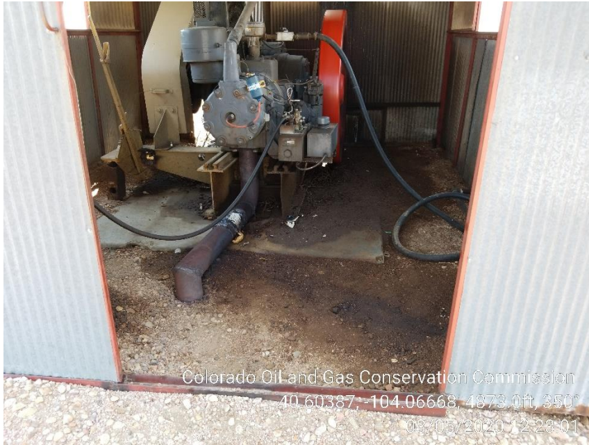
Photo 7 – Stained Soil at Engine
