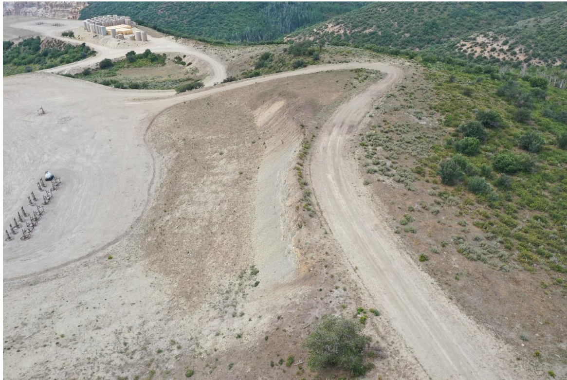
Photo 21: Aerial photo taken from the northeast of the Location, facing southwest. Photo shows cut slopes. Interim areas have not been contoured/regraded and reclaimed to their original condition.
