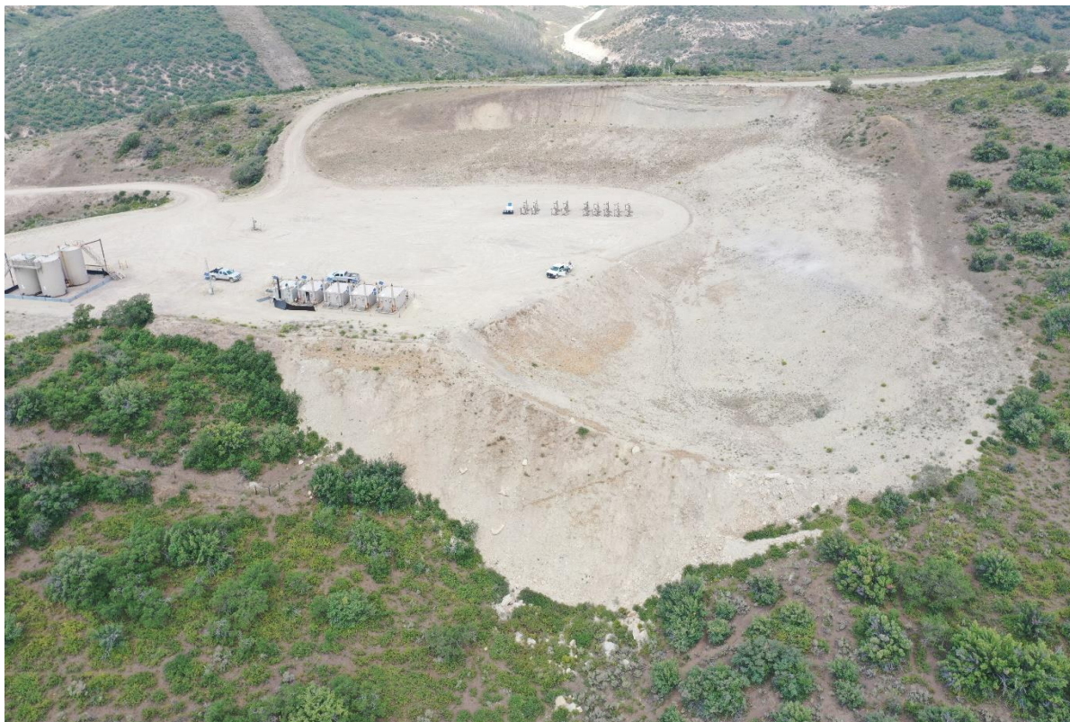
Photo 9: Aerial photo taken from the south of the Location, facing north. Photo shows areas of the Location, including fill slopes, that have not been recontoured/regraded or reclaimed to their original condition in accordance with 1003 rules. BMPs appear insufficient or missing to stabilize slopes and prevent sediment transport.
