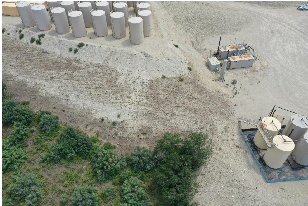
Photo 20: Aerial of the west end of the Location. Photo shows areas of erosion degradation. See photos 10, 11
