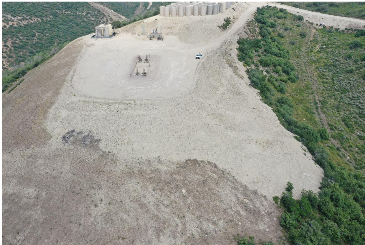
Photo 19: Aerial photo taken east of the Location, facing north. Photo shows overview of the Location and fill slopes; BMPs missing or insufficient to stabilize slopes and/or prevent sediment transport
