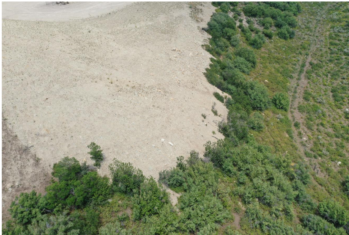
Photo 18: Aerial photo taken east of the Location, facing north. Photo shows overview of the Location and fill slopes; BMPs missing or insufficient to stabilize slopes and/or prevent sediment transport
