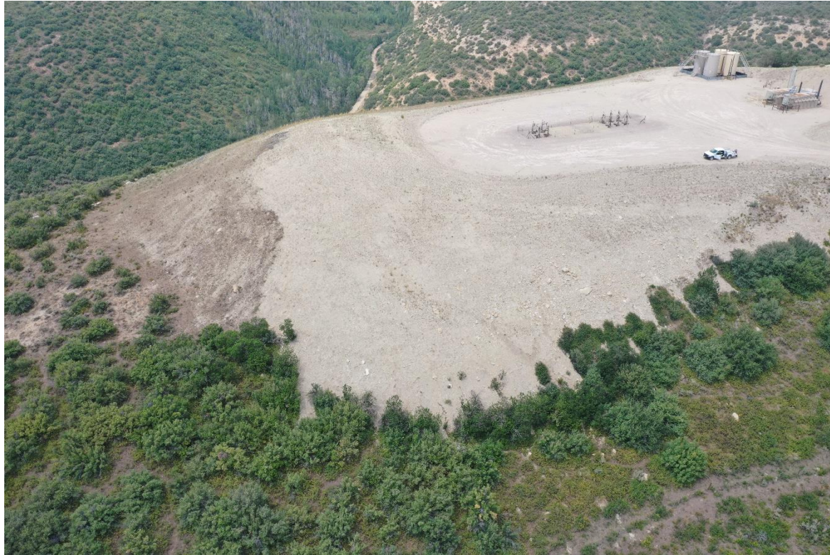
Photo 17: Aerial photo taken east of the Location, facing west. Photo shows overview of the Location and fill slopes; BMPs missing or insufficient to stabilize slopes and/or prevent sediment transport
