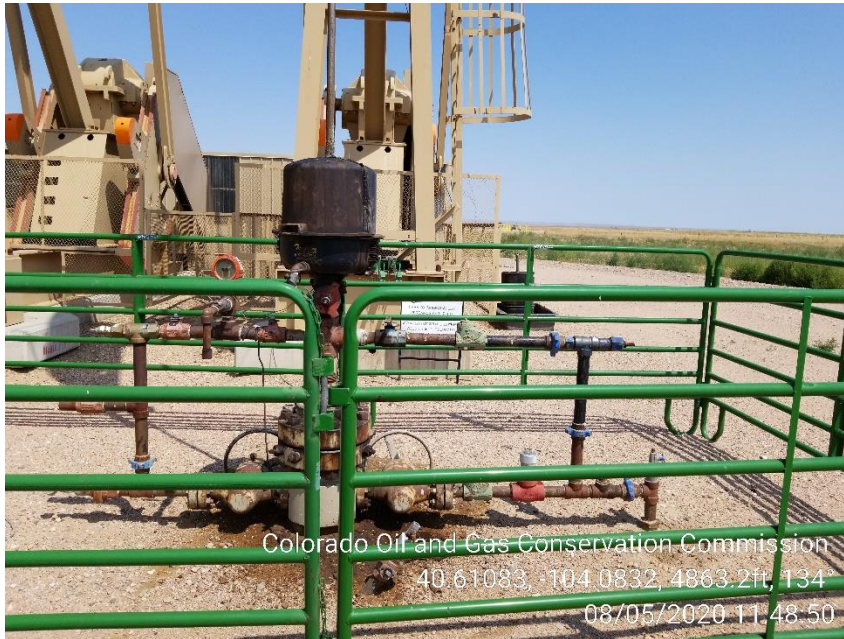
Photo 5 – Stained Soil at 4-3-7-60 Wellhead
