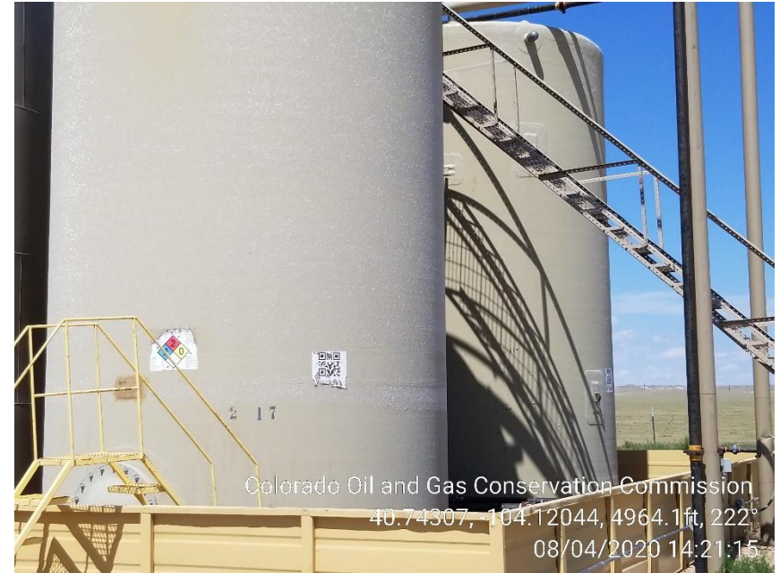
Photo 6 – Southwest Water Tanks – Missing Content and Capacity
