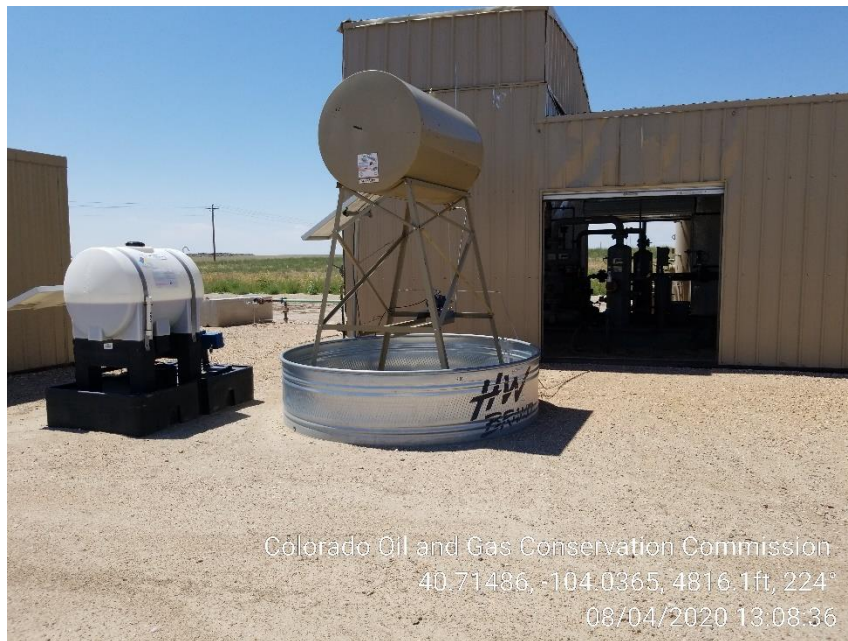
Photo 9 – Methanol Missing Wildlife Netting
