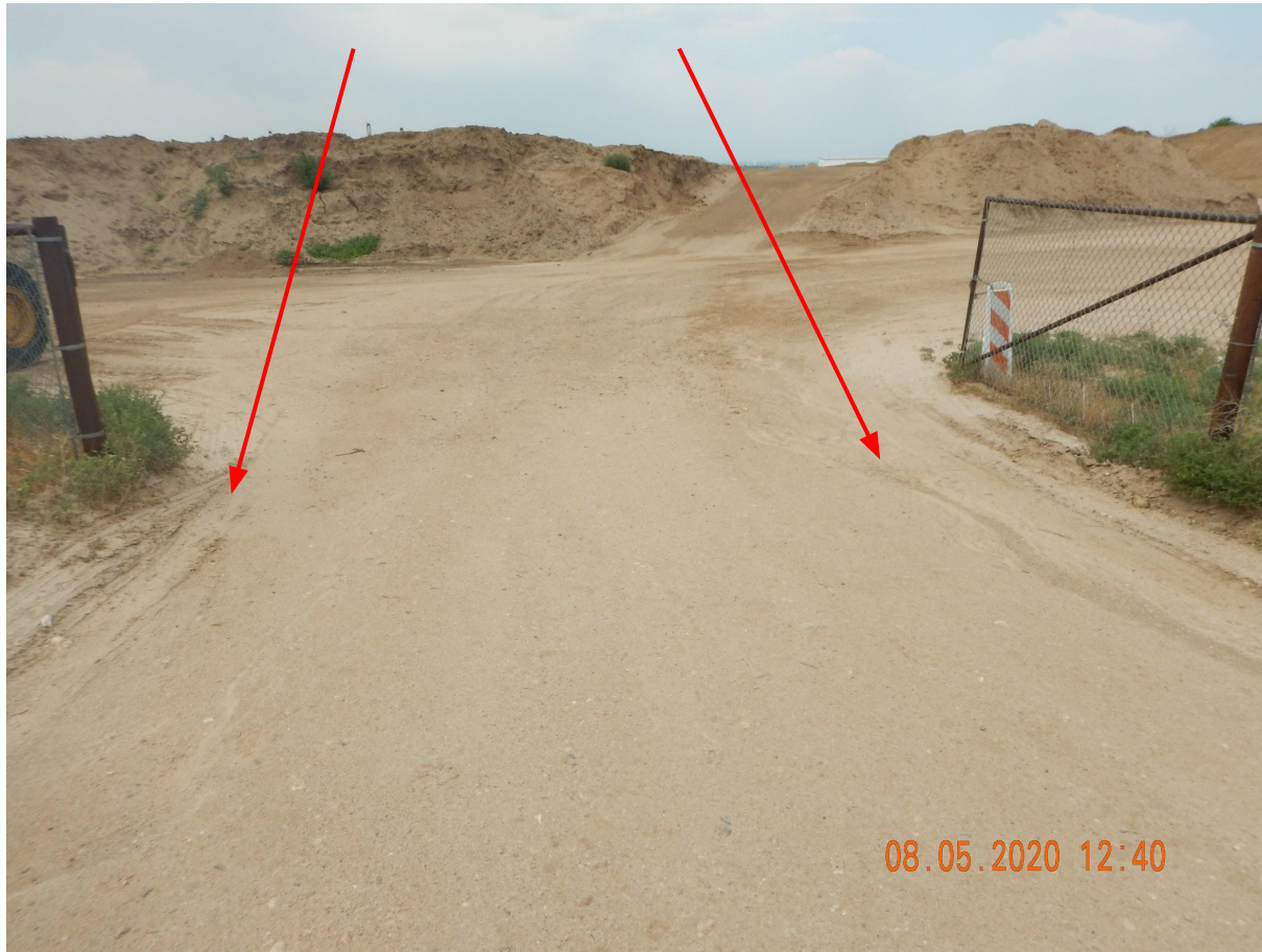
Photo 3. Photo taken from the main point of access to the facility, facing West. Photo illustrates unmanaged stormwater run-on onto the facility.
