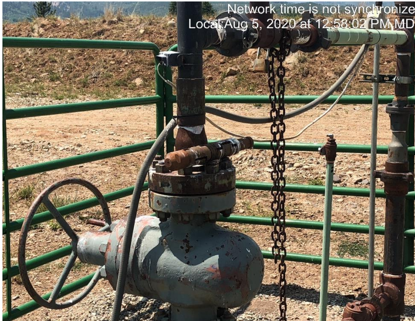
Photo #1683 Unused plunger on wellhead.
