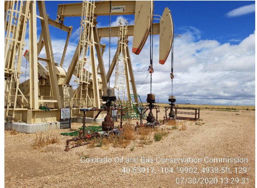
Photo 2 – Pumping Units, Weeds at Wellhead
