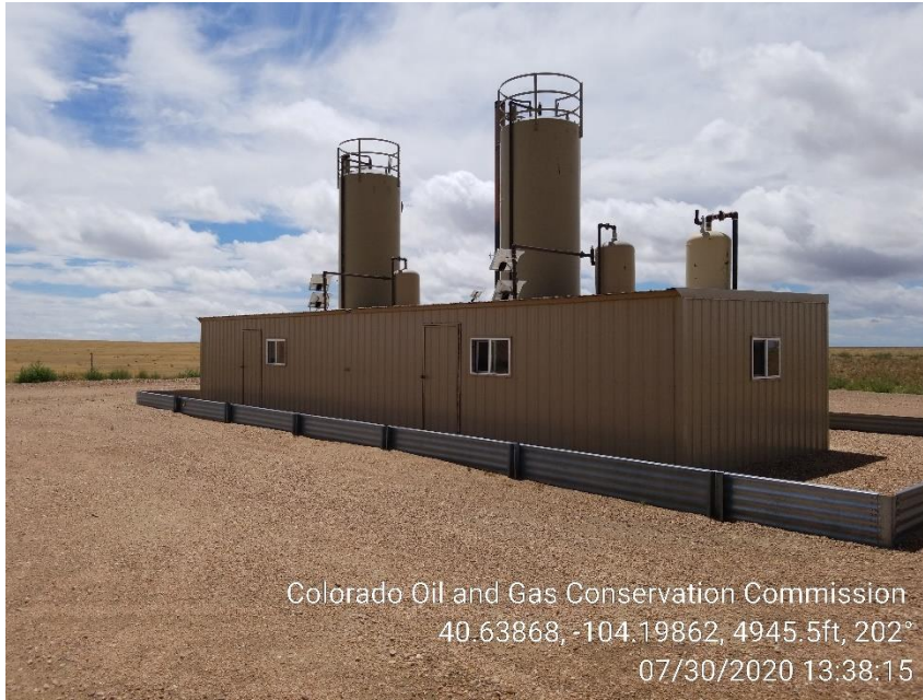
Photo 5 – West Heater Treater
