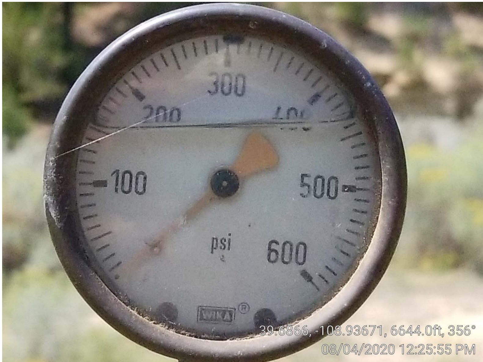
Photo 5. Tubing gage @ 0 psi.
