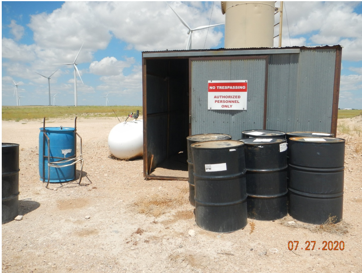
Photo # 4 – Multiple drums stored with no spill containment
