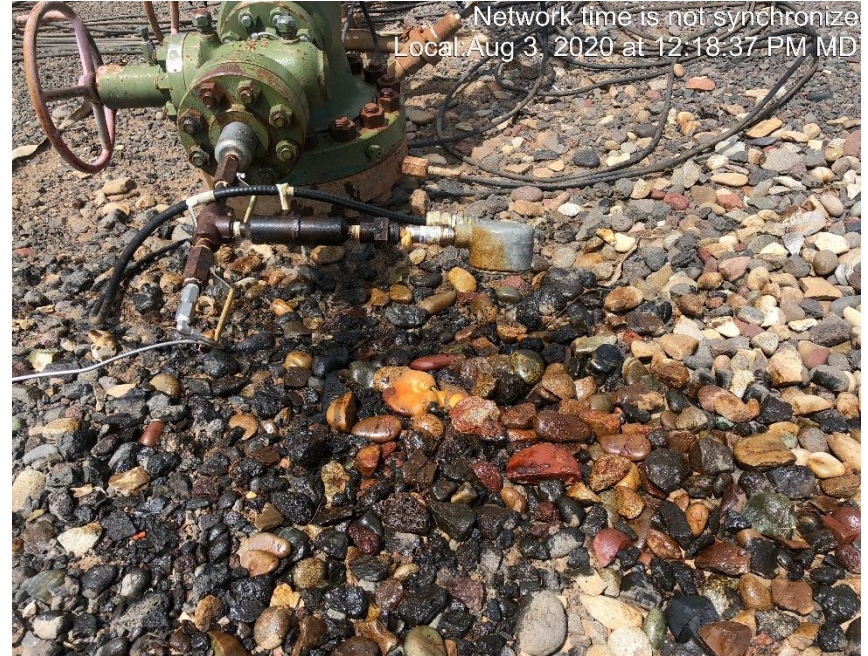
Photo #1661 Gipp 18-14 wellhead leaking at the casing pressure transducer.
