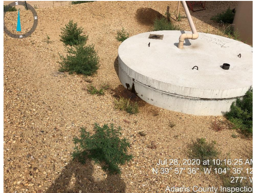
Photo #8 stained soil next to produced water tank.
