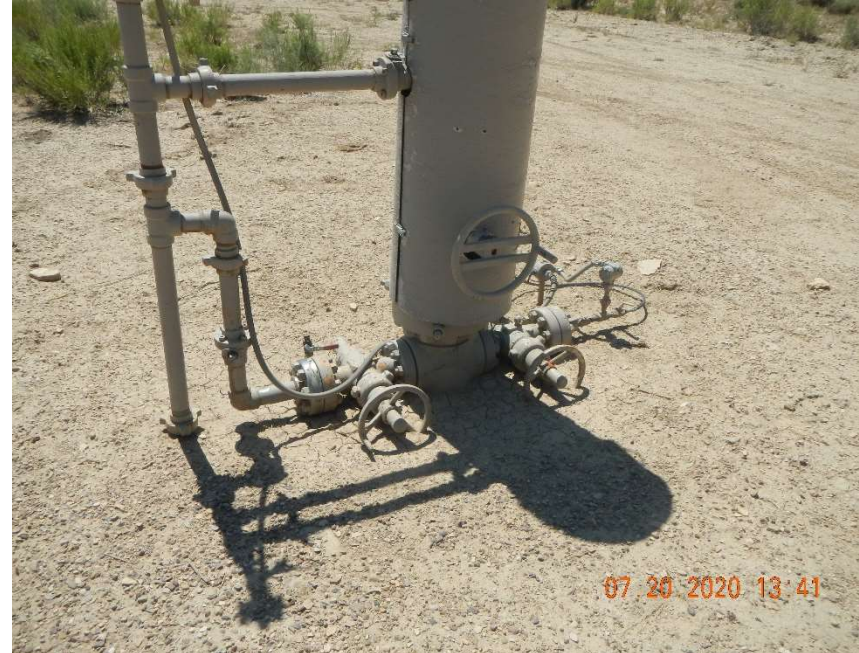
Photo - Wellhead where the audible leak was discovered.
