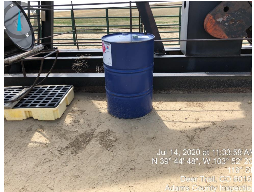
Photo#2 Corrective Action barrel need to be in secondary containment.
