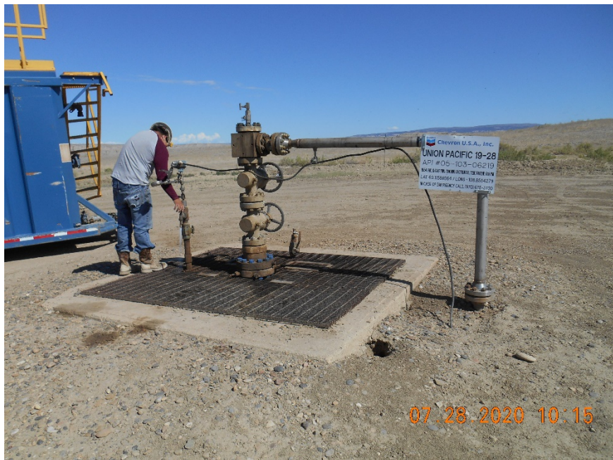
Injection wellhead
