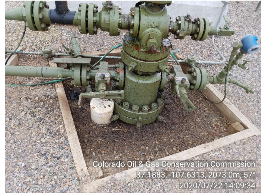
PHOTO 6: PHOTO 4: Approx 2' x 2' area of stained soil/gravel around base of STATE CD 1 wellhead. Clean-up and dispose of stained soil/gravel per Rule 1102.f.(2) and Rule 907.e. CA DATE 8-12-20.
