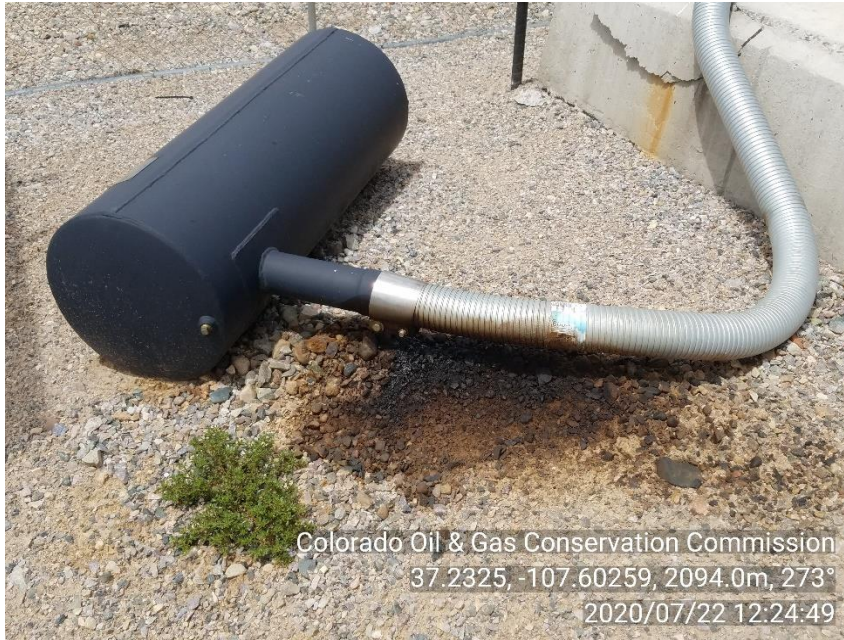
PHOTO 3: Natural gas powered engine exhaust is staining soil/gravel around area of muffler.
