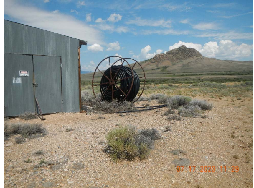
Photo 2. Coil tubing stored on location.
