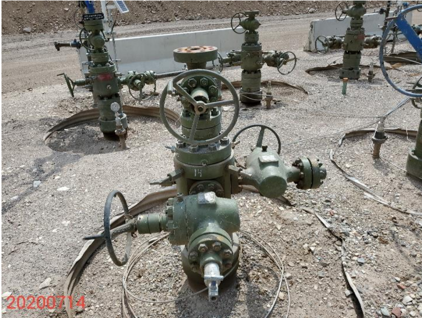
Photo 9: Photo is example of several wells on the Location missing signage.
