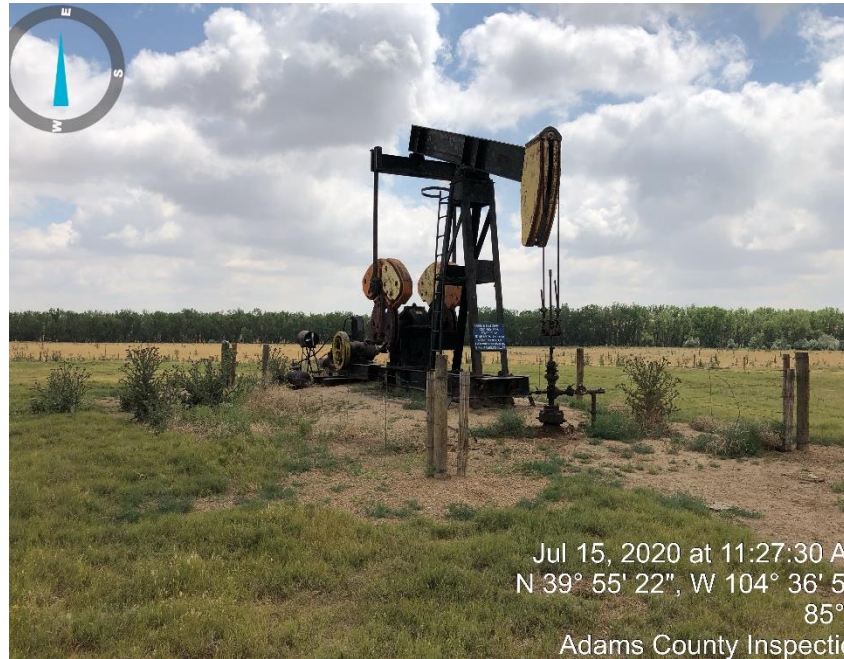
Photo #1 Pump Jack.
