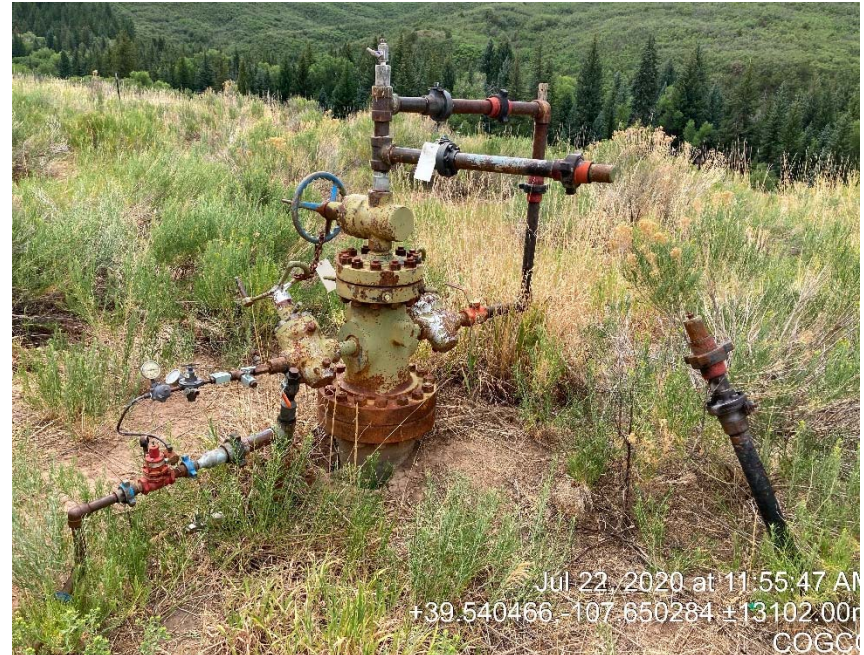
location/weeds/unmarked flow line/wellhead missing sign
