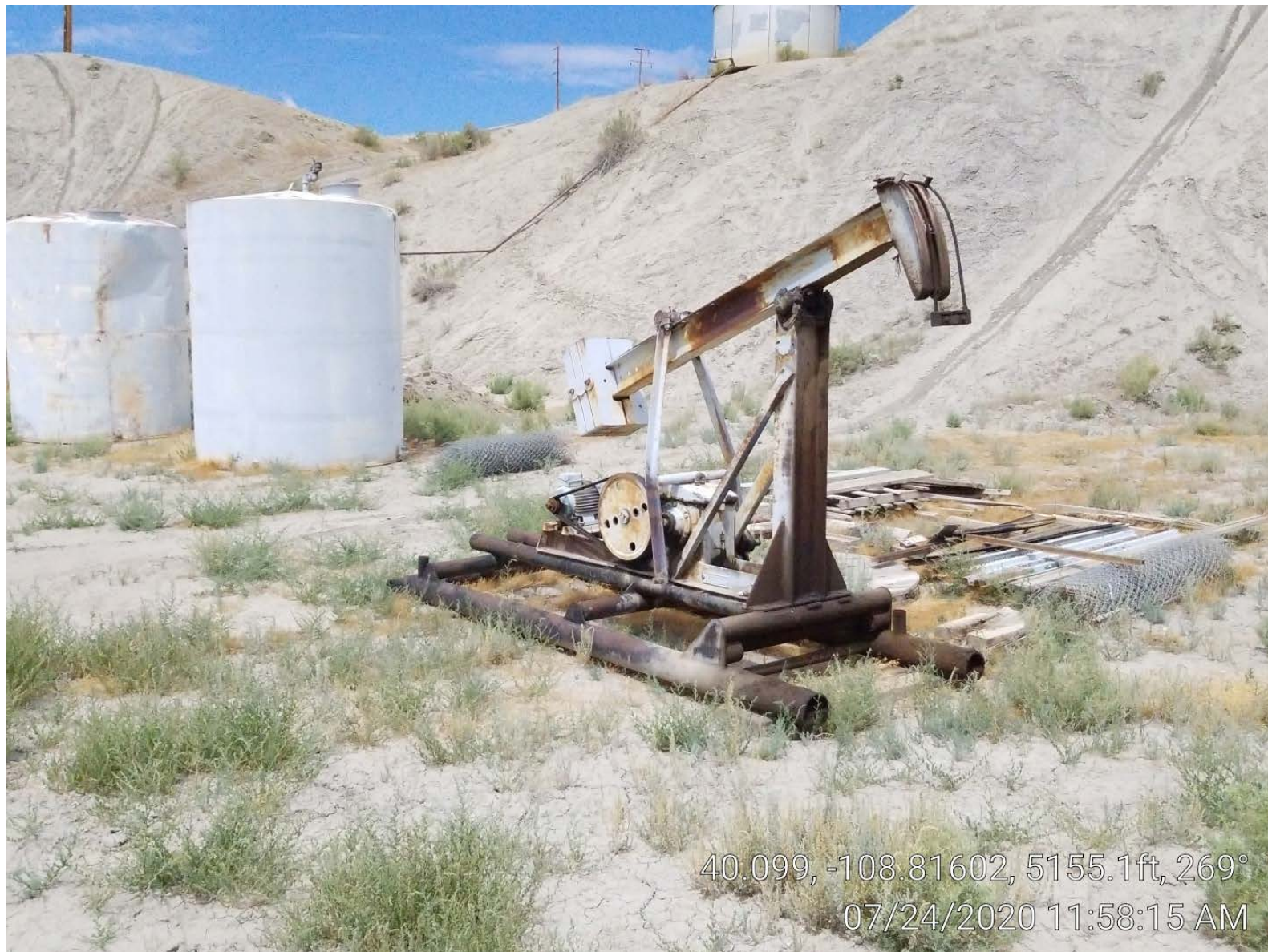
Photo 3. Pump jack from well & unused tanks.
