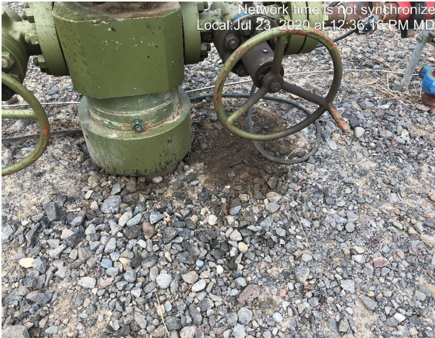
Photo #1596 Multiple places with stained soils by wellheads.
