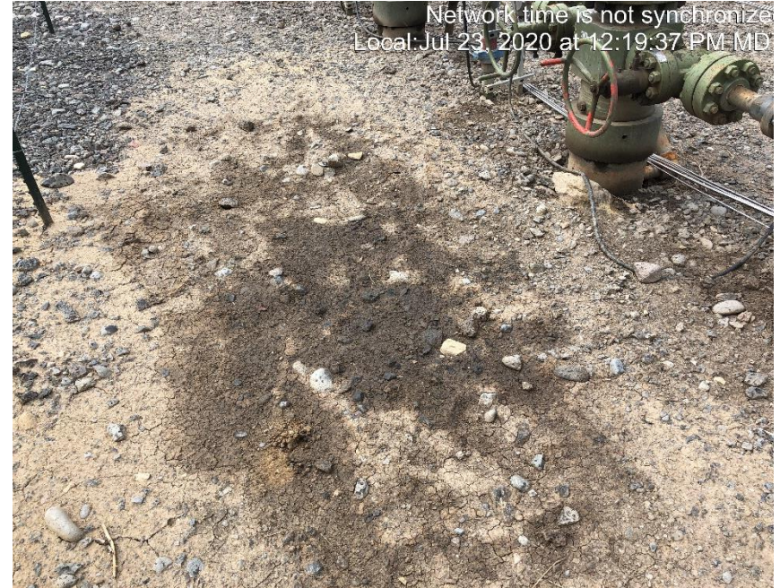
Photo #1593 Multiple places with stained soils by wellheads.
