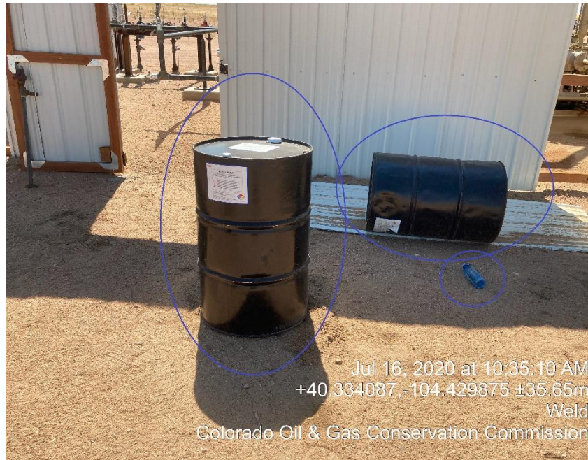
Photo #29 Needs secondary containment/ Trash
