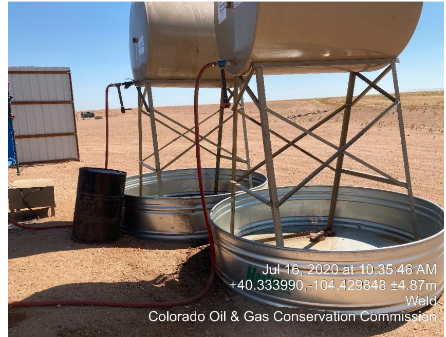
Photo #26 Inadequate wildlife protections (netting) of secondary containments.
