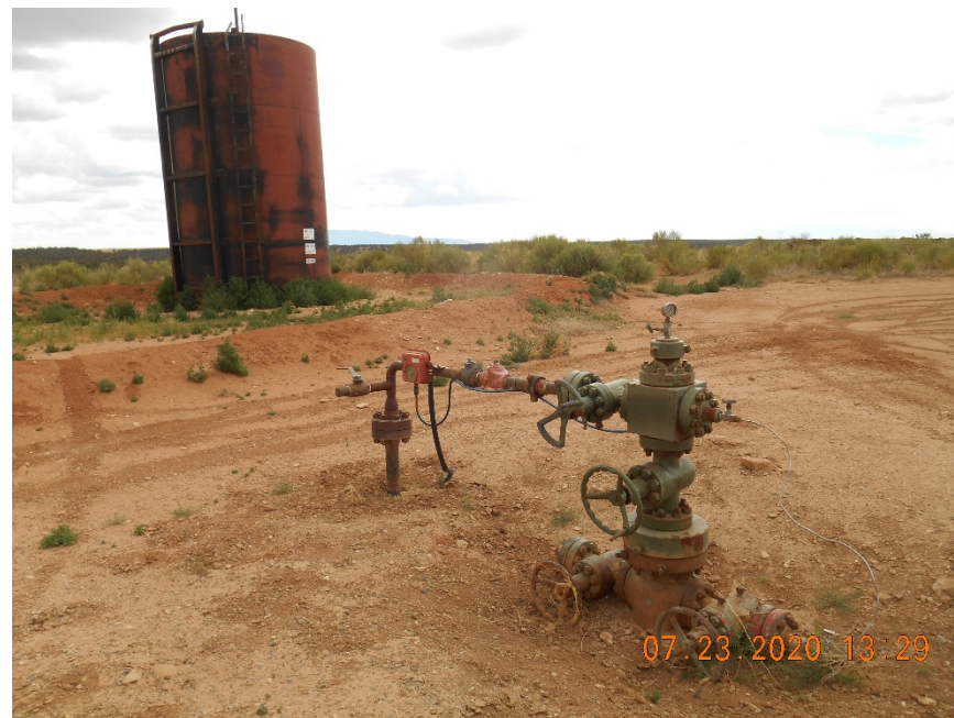
Injection wellhead. Tank Battery.
