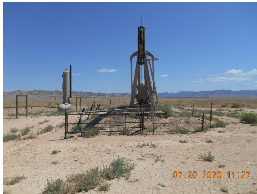
Wellhead with pump jack, fence and sign
