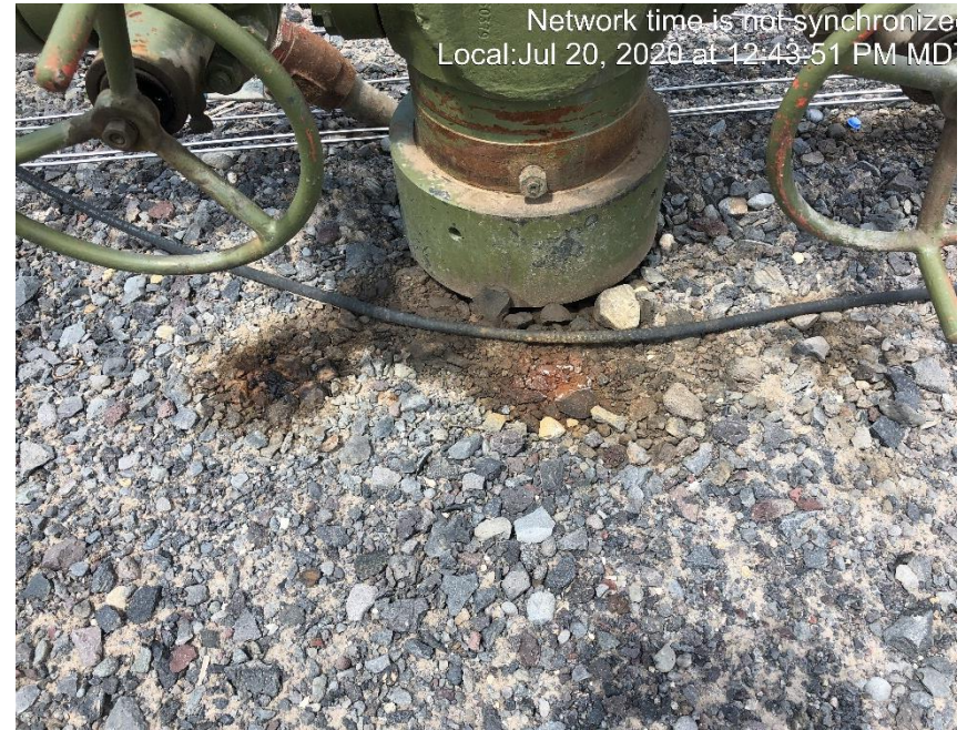
Photo #1563 Multiple places with stained soils at wellheads.
