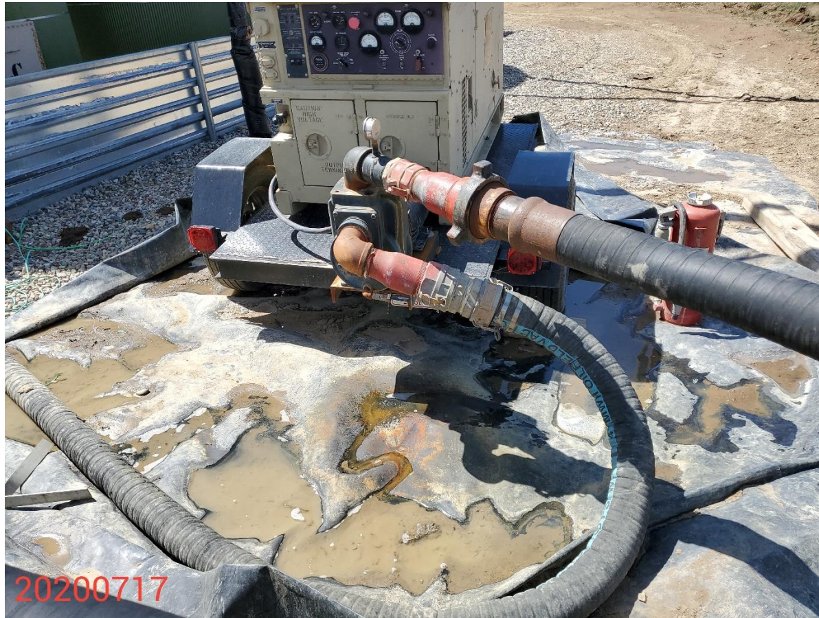
Photo 7: Photo of portable pump and the leaked produced fluids. Photo also shows liner placed under the equipment. BMP insufficient to contain spill .
