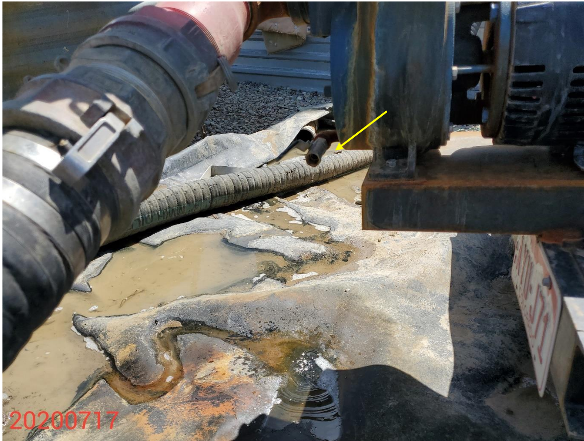
Photo 6: Photo of valve on the portable pump resulting in produced fluid discharge.
