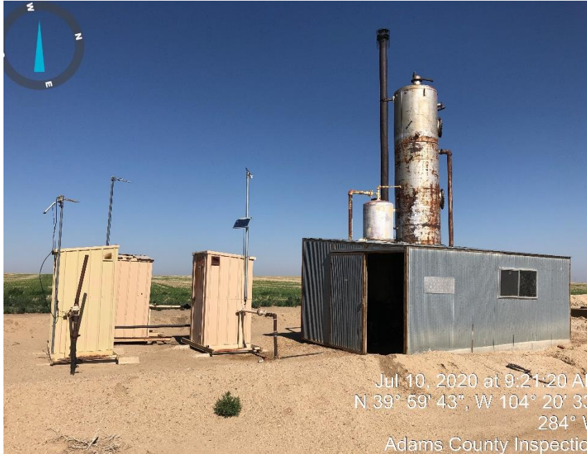
Photo #3 Meters, Separator & treater
