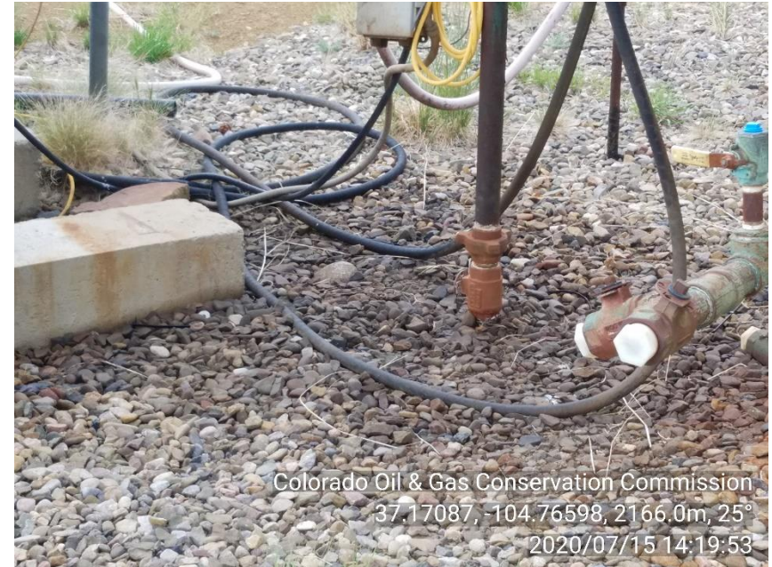
PHOTO 6: AREA OF STAINED SOIL AROUND ENGINE SKID BETWEEN WELLHEAD AND ENGINE SKID. Conduct maintenance on equipment, cleanup stained material and review self inspection processes. COMPLY WITH RULE 1002.f.(2).D. CA DATE 7-22-20.
