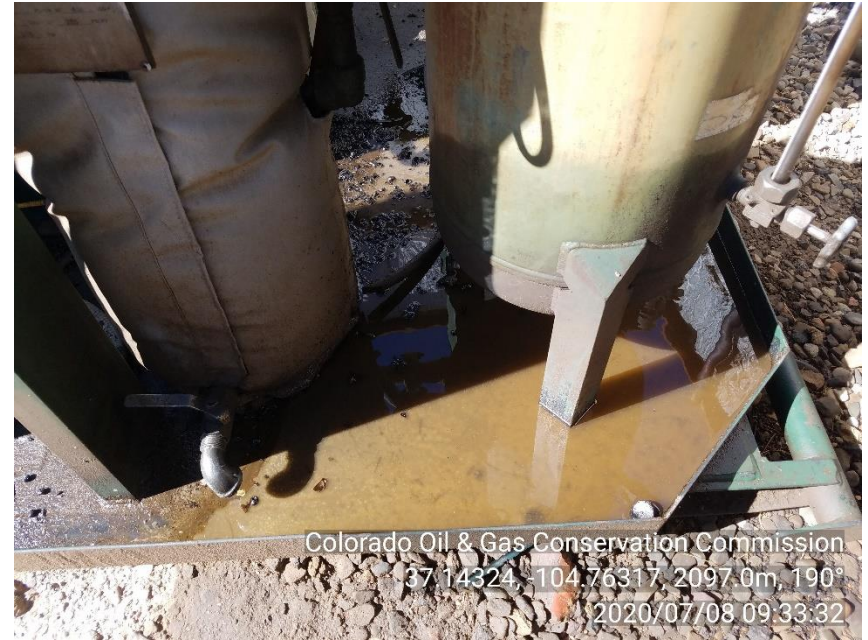
PHOTO 4: STANDING OILY FLUID IN COMPRESSOR SKID. Comply with general provisions of the oil and gas act for wildlife protection. CA DATE 7-20-20.
