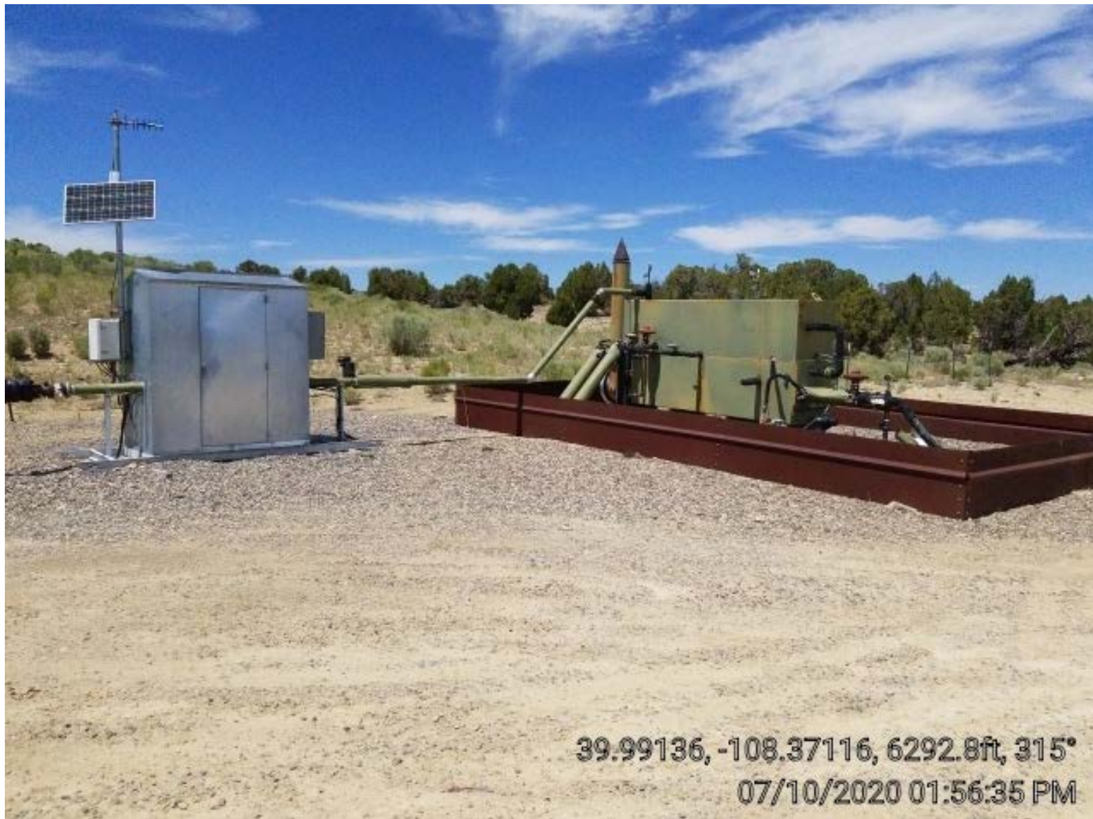
Photo 3. Meter building & separator.
