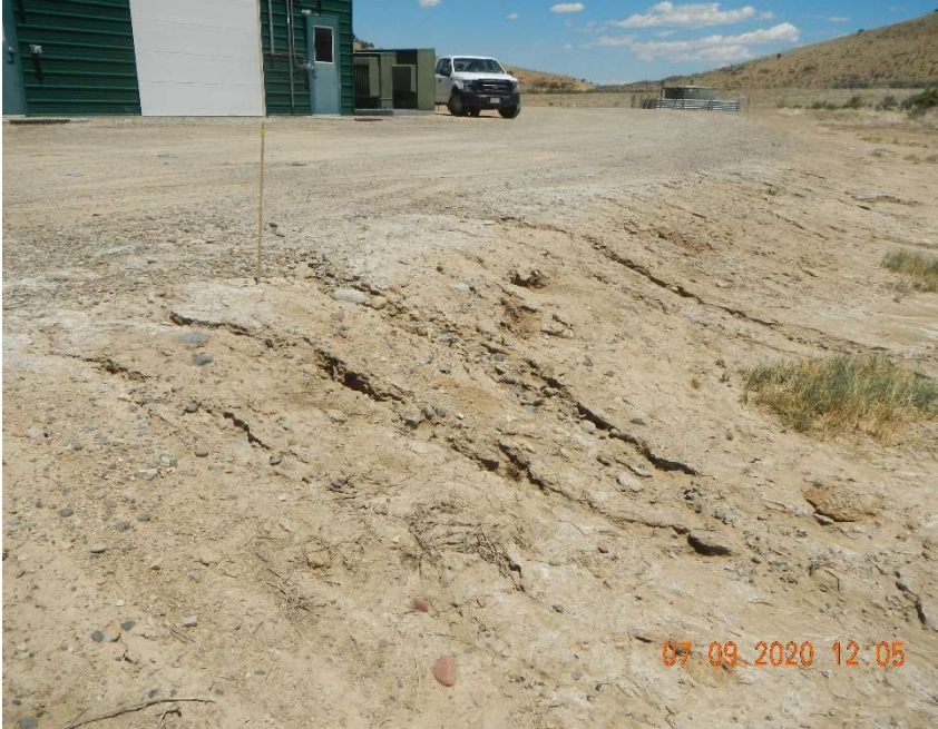
Erosion rills potentially created by the spill/release
