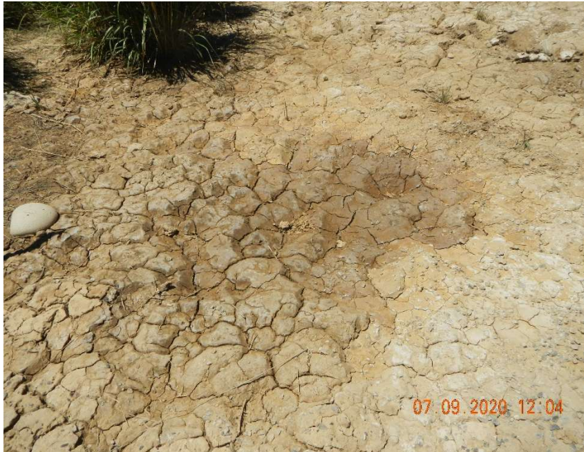
Mud cracks and moist soil where the fluids appeared to have pooled
