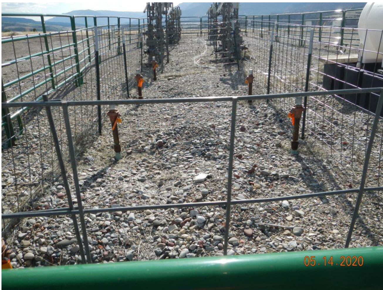
Photo#1: Unused equipment on location: flowlines & Risers.
