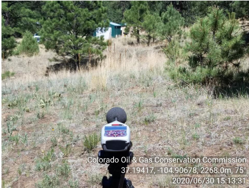
PHOTO 3: SOUND METER SET 350' TO THE WEST BETWEEN LOCATION AND COMPLAINTANTS HOUSE.
