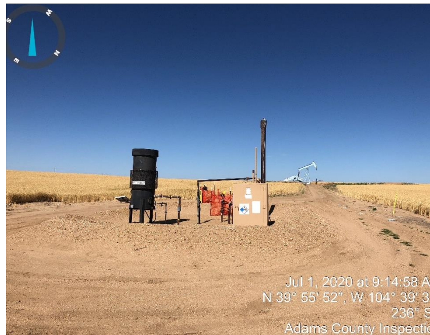
Phot #2 Separator and ECD.
