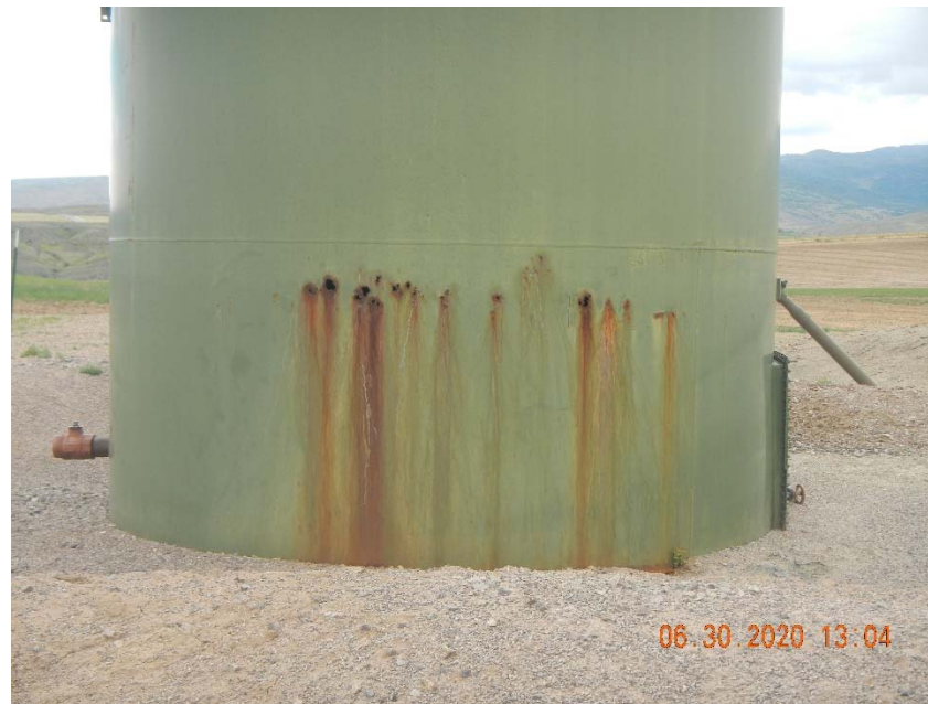
Photo 3. Holes in tank.
