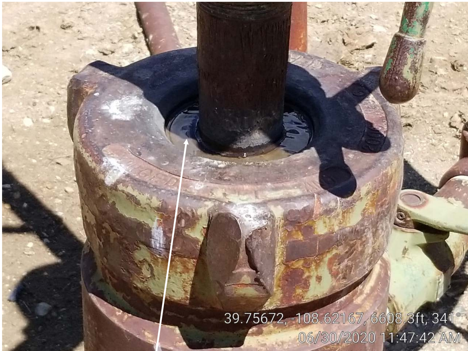
Photo 5. Well. Minor gas leak.
