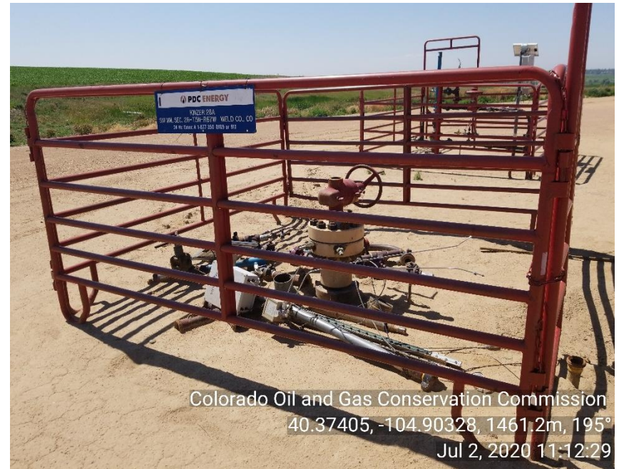
Photo 2: Wellhead; UNUSED/DISCONNECTED EQUIPMENT
