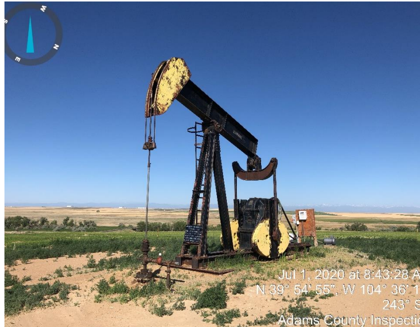
Photo #3 pump jack
